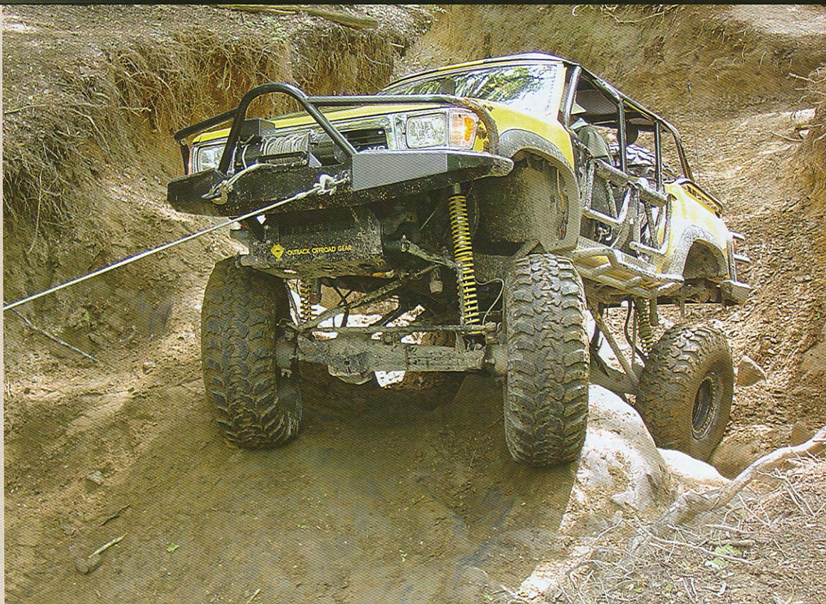
Sometimes even the ARB Air Lockers can't defeat the slick Midwest mud and the winch rope comes out. This shot also gives us a chance to see the Outback Offroad Gear front bumper, made of 3/16" plate and .134 wall tubing. Clean and strong.
